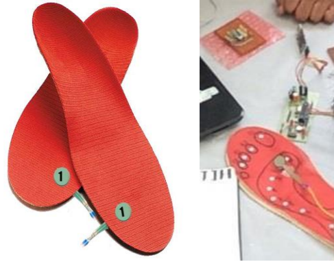
Figure 3 Single FSR placed foot insole (First design prototype)
