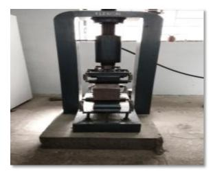
Figure 5 Prism subjected to third point loading method
