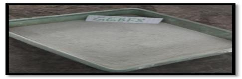
Figure 1 Ground granulated blast furnace slag
