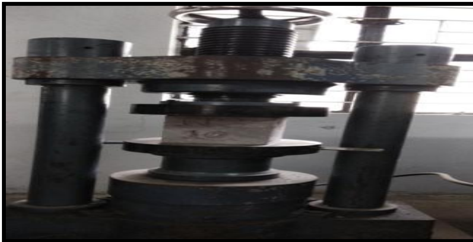
Figure 1 Flexural-testing of specimen
