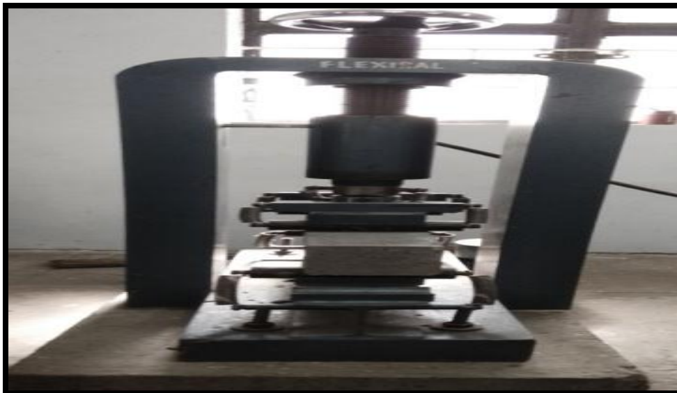
Figure 3 Flexural-testing of specimen
