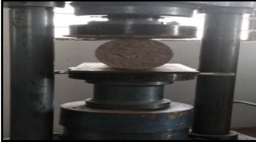
Figure 2 Split-tensile strength of specimen
