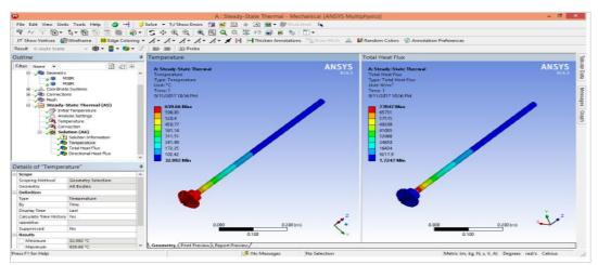
Figure 5 Temperature and total heat flux analysis of graphite stir and steel rod
