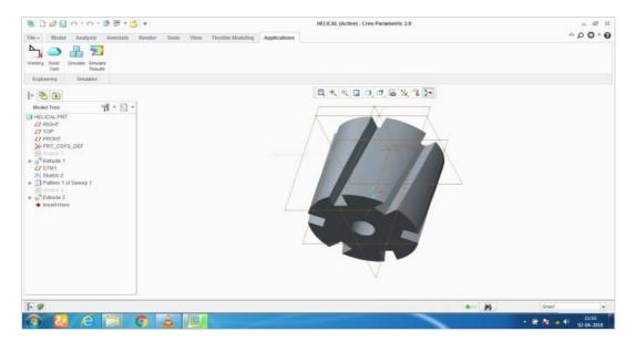
Figure 6 Design of helical type stirrer
