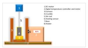
Figure 1 Overall machine setup
