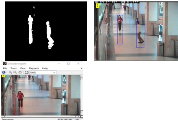
Figure 1 Shows (a) original frame (b) Foreground Detected (c) Clean Foreground after noise removal (d) Detected objects (e)Real Time object detection video play CAVIAR [11] database sample (indoor)
