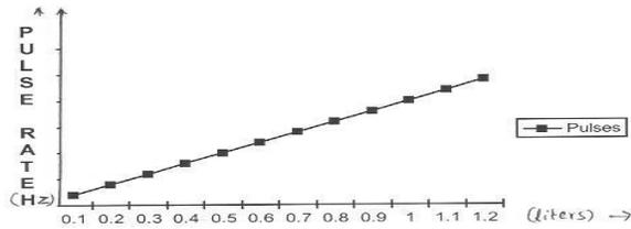
**Fig. 4: Flow Vs Pulse rate**
