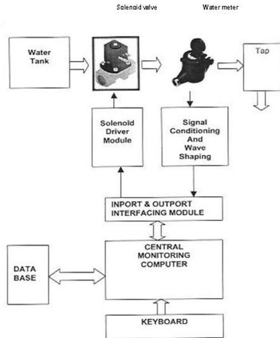
**Fig. 2a: Single Channel Water Metering System**
