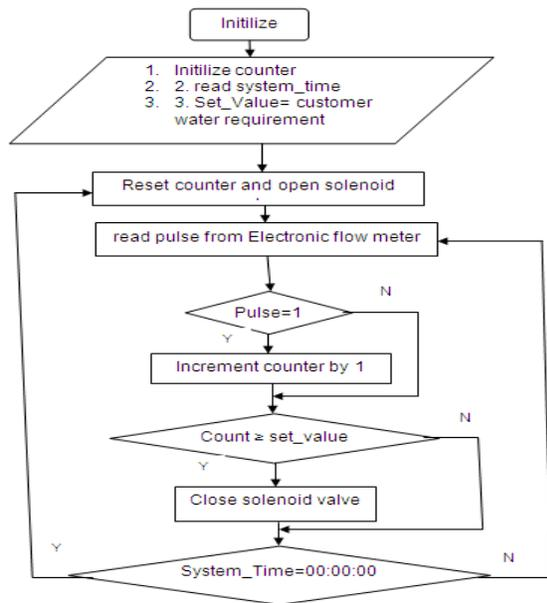
**Fig. 5: Software flowchart for closed loop water metering**
