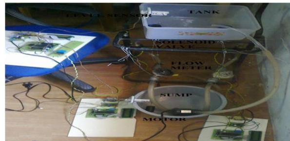
**Fig. 2b: Single Channel Water Metering System**
