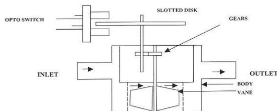
**Fig. 3: Modified Electronic Water Meter**
