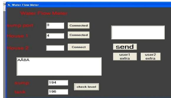
**Fig. 6: GUI of the water metering system.**
