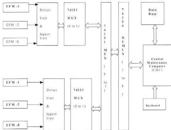
**Fig. 1: Conceptual design of closed loop watering system for multiple users**
