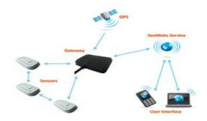
Figure 3: Wireless Mesh Network (WMN)
